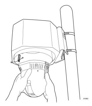
c. Line up the green and red tabs with the green and red labels. Push in on the tabs. Insert the side with the green tab, and then the side with red tab. Continue pushing on the ends of the tabs until both sides click into place.
